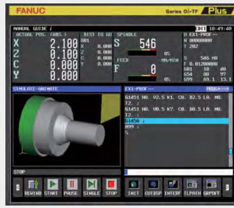
Check cutting result using cutting simulation
