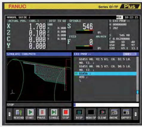
Check cutting path using cutting simulation
